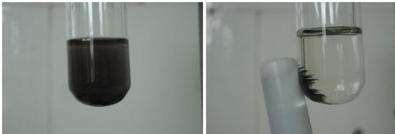
Figure-5 Catalyst nanoparticles in reaction (left) and its separation by simple magnet (right)
